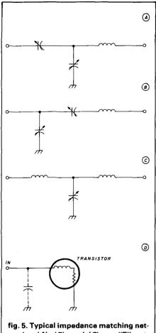
works. (A), (B), and (C) are "T" networks. Value selection is discussed in text. (D) illustrates conversion from series to parallel equivalent circuit on transistor input as explained in text.
